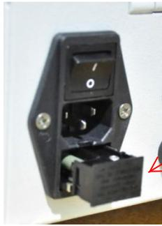
Open the drawer and flip it to the desired voltage so that the arrow on the drawer aligns with the arrow on the frame.
