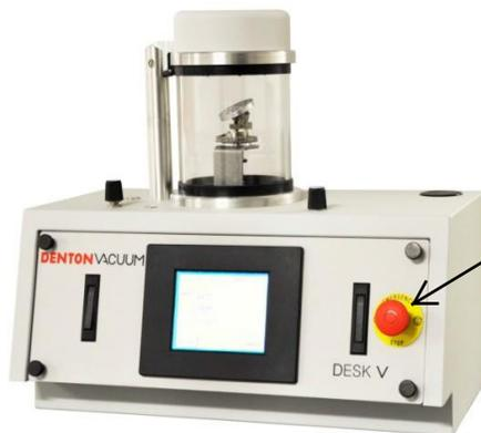
To ensure proper operation, make certain that the emergency button (shown here) is pulled-out completely. The Desk V cannot operate when the emergency button is pushed-in.
