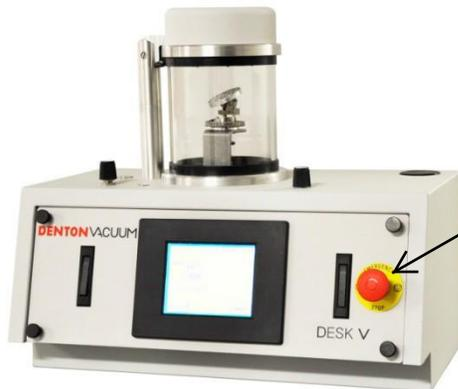
To ensure proper operation, make certain that the emergency button (shown here) is pulled-out completely. The Desk V cannot operate when the emergency button is pushed-in.
