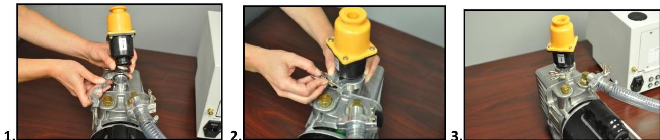
Check oil level in the mechanical pump. If the oil level is  $\frac{1}{2}$  full in the sight glass, the pump is ready. For detailed instructions, refer to the Maintenance section of this manual.
